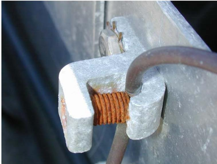
An example of improper component selection and subsequent galvanic corrosion during nine months of outdoor service.
